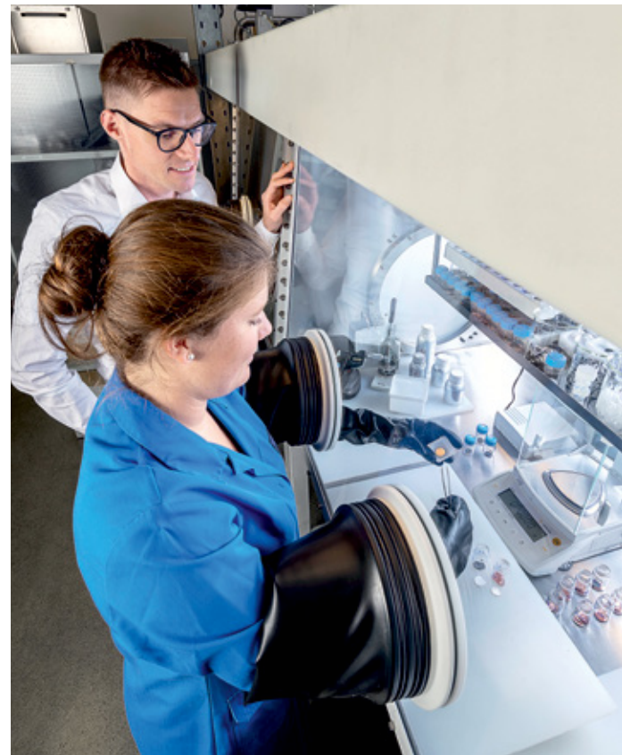
↑ Glove-box for cell building. In our laboratory we produce cells for testing according to standard and customized protocols
